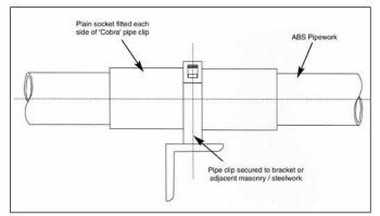
1. Small Bore (up to 4" Pipework)
