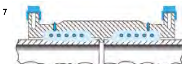
Melt pressure reaches optimum value at end of energising cycle. Emergence of the melt at the indicator holes shows that fusion is complete.
